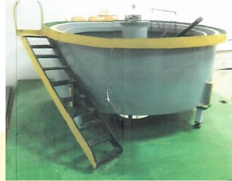
Figure 14 Model for a circular Sedimentation Tank
